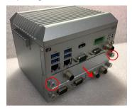
Step 3 Fasten the SSD screws (marked by the red arrows below) to fix the SSD. Then screw the SSD firmly to the tray (marked by the yellow circles) and install the tray back to the system.
