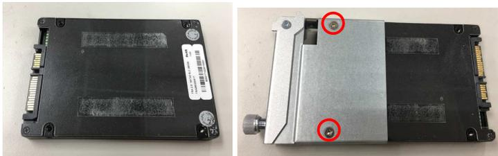
**Step 2** Install the SATA drive into the slot and fasten the screw to lock the SATA drive to complete the installation.
