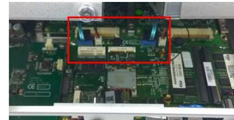
**Step 4** Loosen below screws to remove the cover and put the thermal pad on the slot.
