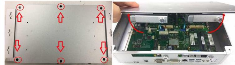
**Step 3** Disconnect the four SATA connectors and remove the bracket.
