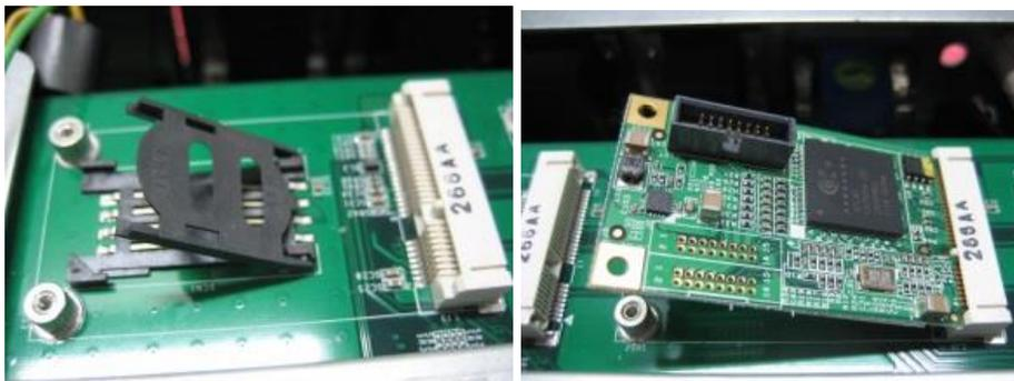
**Step 2** Fasten the screws to complete the installation.
