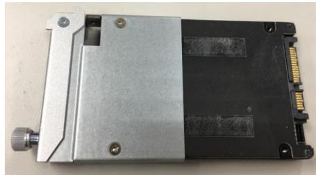
**Step 3** Install the SATA drive into the slot and fasten the screw to lock the SATA drive to complete the installation.
