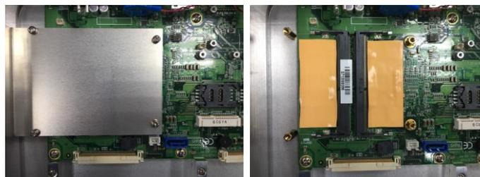
**Step 4** Install the DDR module with caution and put the thermal pad on the DDR module again. Then screw the DDR cover to finish the installation.
