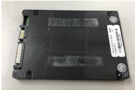
**Step 2** As shown in the picture, slide the HDD/SSD into the SATA tray. Insert screws into each side of the SATA drive through the corresponding holes.
