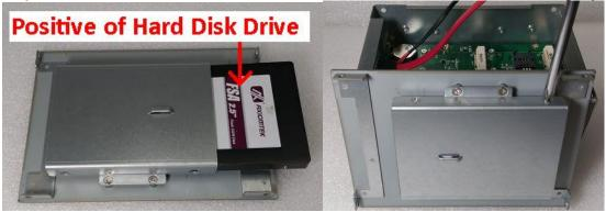
Note: The positive of Hard Disk Drive must be upward when insert the Hard Disk Drive into the bracket.
