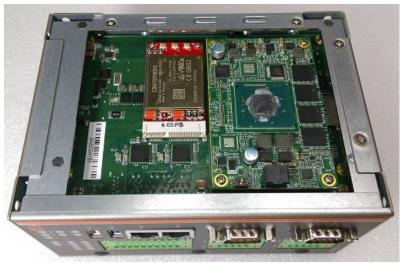
Step 6 Plug the SIM card into the SIM slot and the positive of SIM Card is as below picture.
