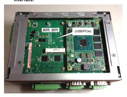
> Two wireless sockets are near SSD cover side, one socket supports mSATA/USB/PCIe interface, another supports USB/PCIe interface only.
