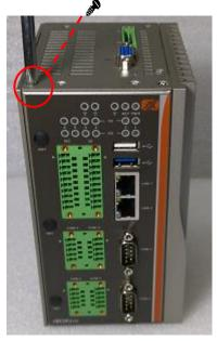
Step 3 Plug the mSATA module in the socket and use screws to fix tightly.
