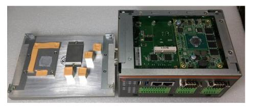
Step 3 Take out the thermal pad form the wireless module kit, then stick on the thermal parts.
