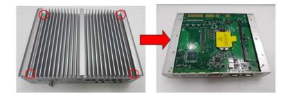
Step 3 Located the dual SO-DIMM sockets on main board.
