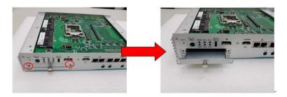
Step 3 Turn the SATA drive tray upside down to install SSD/HDD and then fasten the four HDD screws to secure the SATA drive tray.
