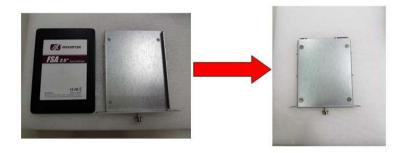
Step 4 Slide the SATA drive tray back into the system and fasten the screws firmly to complete the installation.
