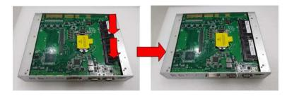
Step 5 Put the top cover back and fasten four screws back onto the system.
