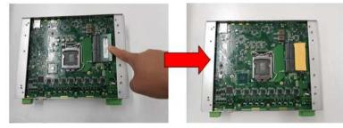
Step 5 Assemble top heatsink with chassis through 4 screws carefully to complete Processor / SO-DIMM installation.
