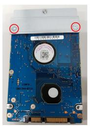
Step 6 Connected the SSD/HDD directly and make sure the insertion is complete.
