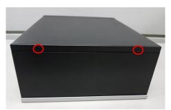
Step 3 Remove the bottom cover and locate SSD/HDD within the red line marked.
