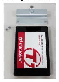
Step 5 Fasten two screws to fix SSD/HDD.
