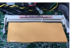
Step 5 Insert the SO-DIMM into the socket and push the module down until it is locked in place by the two end latches.
