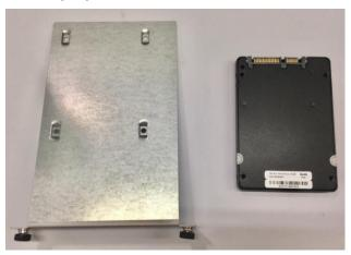
Step 5 Fasten four screws to fix HDD/SSD.
