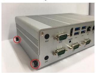
Step 3 Pull out the HDD/SSD drive bay bracket.
