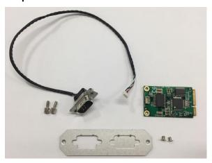
Step 5 Assemble CAN Bus connector with bracket.
