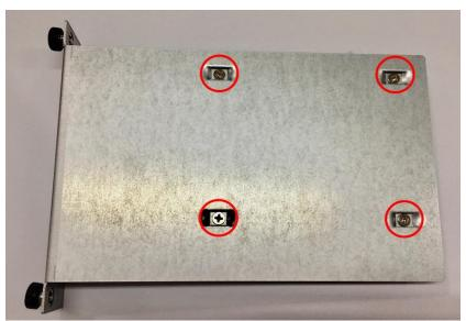
Step 6 Connect the SSD directly and make sure the insertion is complete and fasten two screws.
