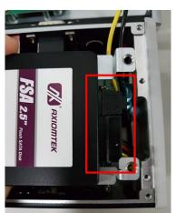
Step 8 Fasten screws of HDD bracket to complete the SSD/HDD installation.
