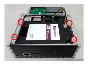
Step 9 Recover and fasten all screws of the bottom cover
