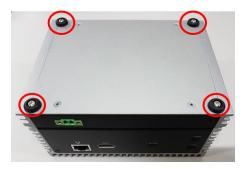
Step 3 Loosen the screws to remove SSD/HDD bracket and then located the Mini PCle slot.
