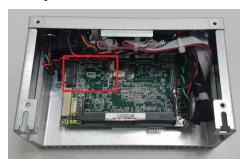
Step 5 Insert the M.2 WiFi module firmly and fasten the screw.
