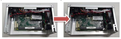
Step 6 Put the bottom cover back and fasten all of screws to complete installation.
