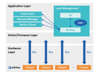
Intelligent AXView 2.0 suite is designed to meet the needs of applications for IoT/M2M. Ranging from physical layer connectivity, communication layer protocol, middleware API, high level software for remote management, store Apps and service cloud are covered.
