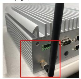
Step 13 Loosen the SIM cover screw and insert the SIM card.
