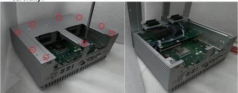
Step 5 Insert the wireless module (3G/4G/BT/GPS module etc.) into the slot with the marking "PCIe / USB".
