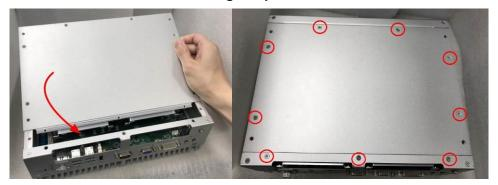
Step 7 Slide the SATA trays back and fasten screws firmly to complete the installation.
