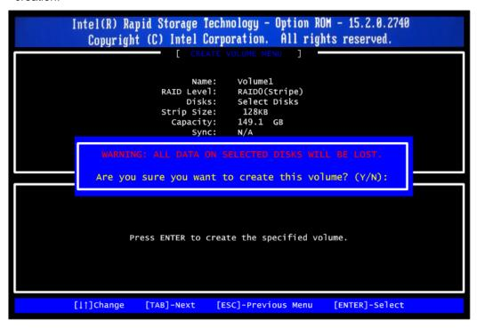
3.8. After the creation is completed, you will see detailed information about the RAID array in the Disk/Volume Information section, including RAID mode, disk block size, disk name, disk capacity, etc.
