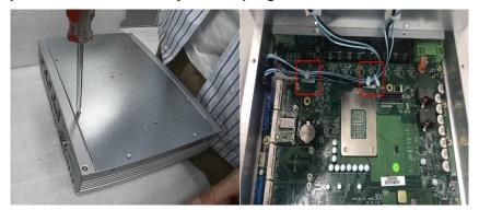
Step 4 Insert the wireless module (3G/4G/BT/GPS module etc.) into the slot with the marking "PCIe / USB". Then fasten the screws as shown.
