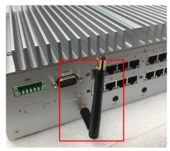
Step 14 Loosen the SIM cover one screw and insert the SIM card.
