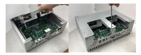
Step 7 Slide the secured SATA tray back and fasten screws tight to complete the installation.
