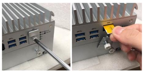
[Note] The system provides two PCle slots for SIM card installation. Pay attention to the orientation when inserting a SIM card: The SIM card's contacts must face downward when the card is being inserted into the SIM1 slot; the card's contacts must face upward when it is being inserted into the SIM2 slot.
