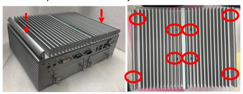
[Note] When removing the top cover to change accessories, the CPU will stick on the underside of the cover. To avoid damaging the CPU by squeezing, please take it down carefully by holding the edges of the CPU and follow section 2.1 to reinstall.
