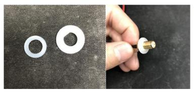
Step 8 Take out the fastening nuts from the 4G/3G kit package (Figure 1). Insert the end of the RF cable through the antenna hole (Figure 2 and 3). Place the smaller gasket and screw it tight (Figure 4) with the fastening nuts.
