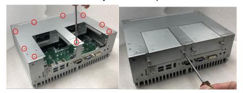
Step 13 Turn the system back to its upright position and screw the RF antenna tight.
