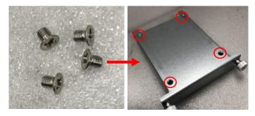
Step 5 Slide the secured SATA drive tray back into the system and fasten the screws firmly to complete the installation.
