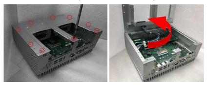
Step 5 Insert the PCIe card and fasten the screws as shown.
