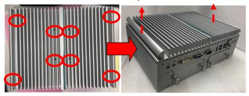
Step 3 Put the thermal pads on the secant locations.
