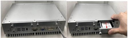
Step 3 Loosen nine bottom cover screws as shown and open the cover carefully
