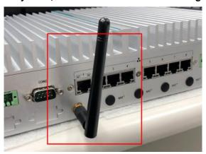
Step12 Loosen the screw to remove the SIM cover and insert the SIM card.
