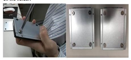
Step 5 Put the drive holders to precisely meet the screws hole positions and tighten screws.
