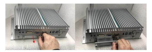
Step 4 Turn the SATA drive tray upside down to install SSD/HDD and fasten the four screws to secure the SATA drive tray.
