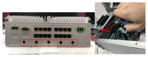
Step 8 Connect the RF cable to the connector of the 3G module marked with "MAIN".
