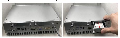
Step 4 Loosen all screws and open the bottom cover carefully.
