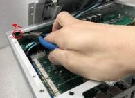
Step 7 Connect the RF cable to the connector of the 3G module with the marking "MAIN".
