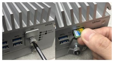
[Note] The system provides two PCle slots for SIM card installation. Pay attention to the orientation when inserting a SIM card: The SIM card's contacts must face downward when the card is being inserted into the SIM1 slot; the card's contacts must face upward when it is being inserted into the SIM2 slot.
