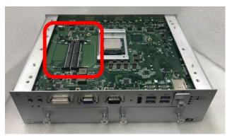
Step 4 Insert the gold colored contact of the memory module into the socket and push the module's two end latches down until locked.
