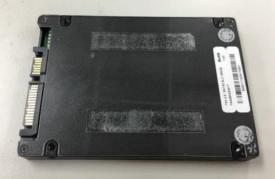
Step 5 Turn the SATA drive tray upside down to install SSD/HDD and fasten the eight screws to secure the SATA drive tray.
