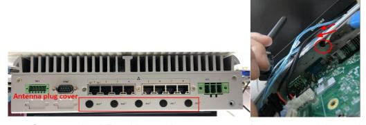
Step 6 Connect the RF cable to the connector of the 3G module marked with "MAIN".
