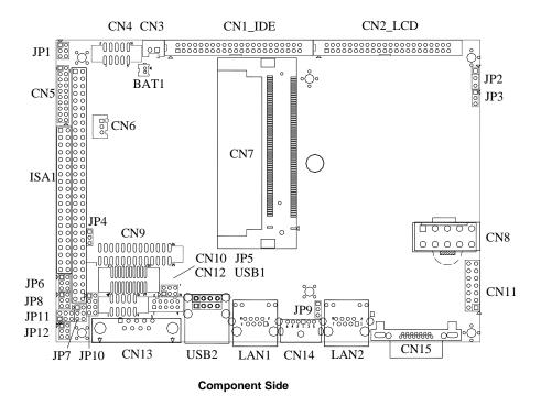
**Note** The Limited Height of Component Side is 30mm.
