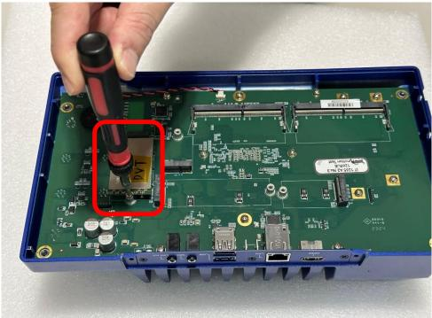
Step 5. Connect the RF cables to the connectors of the 5G/LTE module. Remove the hexagonal metal screw.
