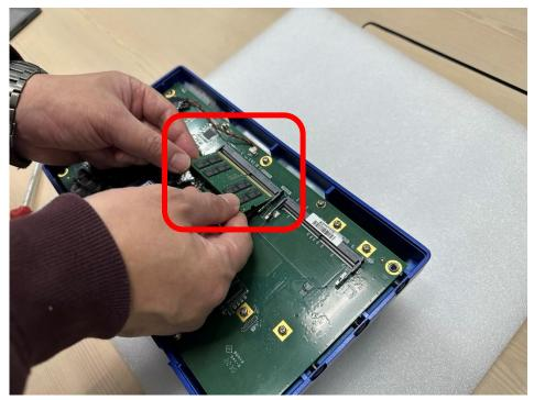
Step 4. Insert the gold-colored contact of the memory module into the socket and push the module's two end latches down until locked.
