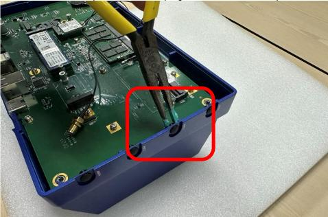
Step 7. Place the RF cable and insert the end of the RF cable through the antenna hole.
