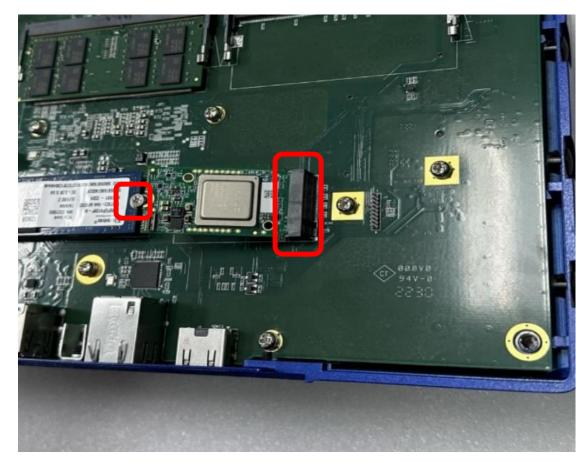
Step 4. Insert the gold-colored contact of the AI module into the socket. Step 5. Fasten the screw as shown.
