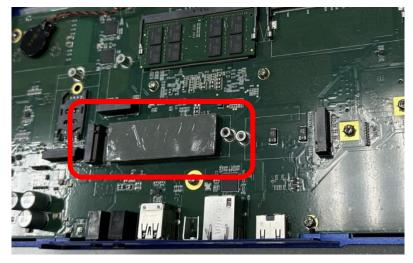
Step 4. Insert the gold-colored contact of the NVMe SSD module into the socket.
