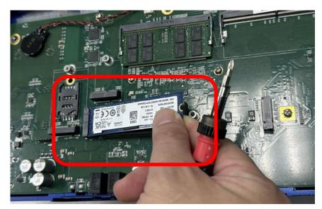
Step 5. Fasten the screw as shown.
