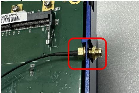
Step 8. Fastening the hexagonal metal screw from the outside as shown.
