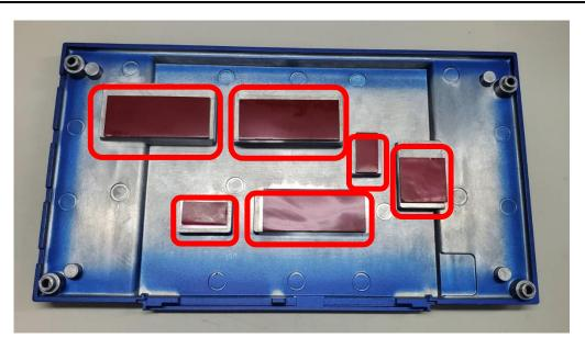
Step 4. Put the thermal pads on the SO-DIMM socket, NVMe SSD socket, AI Module socket.
