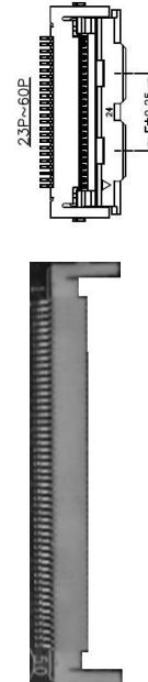
This board also has a 40-pin ZIF connector (CN2) for interfacing TTL LCD to baseboard.
