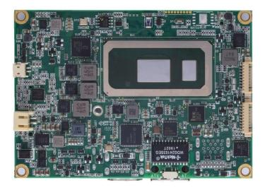
The PICO52R is a Pico-ITX board with the 8<sup>th</sup> Generation Intel<sup>®</sup> Core<sup>™</sup> i7/ i5/ i3 and Celeron<sup>®</sup> processors that deliver outstanding system performance through high-bandwidth interfaces, multiple I/O functions for interactive applications and various embedded computing solutions.
