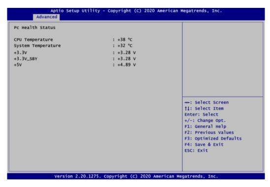
This screen displays the temperature of system and CPU, system voltages (+3.3V, +3.3V standby and +5V).
