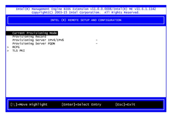
1. Select TLS PKI to get into remote configuration screen. Then select Start Configuration to activate it.
