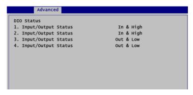
If DIO Modification is enabled, you can load manufacture default and access to the DIO status sub screen to change inputs/outputs setting, see images below.
