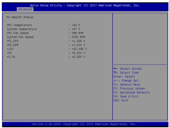
This screen displays the temperature of system and CPU, cooling fans speed in RPM and system voltages (VCC\_CPU, VIN1~VIN4 and VBAT).
