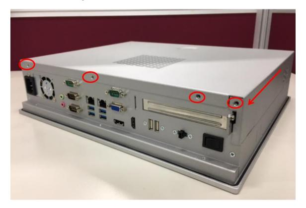
Figure 2-1 Remove Back Cover of the P1157E-500
