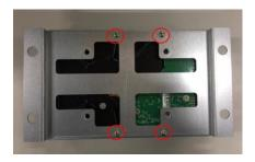
▲ Fix 3.5" HDD on the back of bracket
