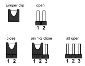
Before applying power to the P1157E-500 series, please make sure the jumpers are in default positions which are defined as follows:
