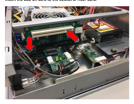
Secure the metal bracket of the card to the system case with two screws. Installations complete. Step 3
