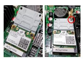
Step 3 Find the built-in Antenna cable and connect it wireless LAN card.
