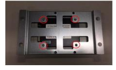
▲ Fix 2.5" HDD on the back of bracket
