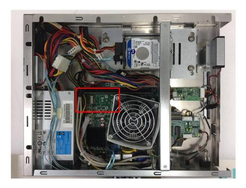
Step 2 Insert wireless LAN module to Mini card slot and fixing it by 1 screw.
