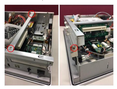
Step 2 Insert the riser card in the socket firmly until it is installed completely. Then insert the add-on card to the socket of riser card.
