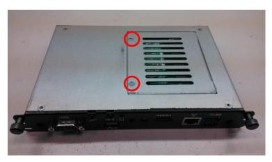
After losing the screws, extract the real of chassis out of the module.
