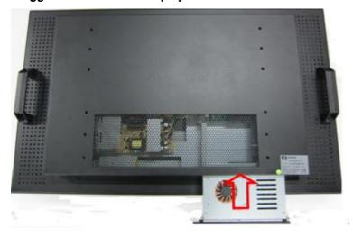
Caution: When plugging OPS880-HM into an OPS display, make sure the module's heat sink is facing outside of the display. Axiomtek is not responsible for any damage caused by wrong installation.
