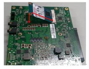
Step 4.2 Install mSATA module. Place the mSATA module into the socket and press it firmly down until it is fully located.
