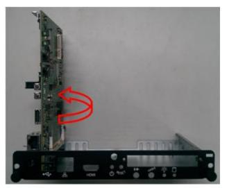
Step 5.2 Install Wi-Fi module. Place the Wi-Fi module into the socket and press it firmly down until it is fully located.
