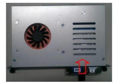
Step 6.3 Plug HDD drive in to HDD connector
