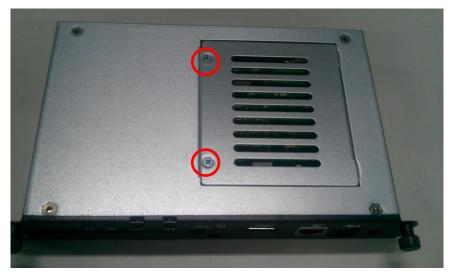
Step 3.2 After losing the screws, extract the real of chassis out of the module.
