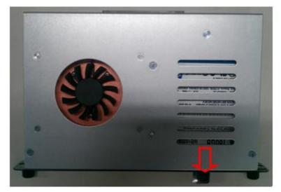
Step 6.4 Pull the HDD Mylar to slot-out the HDD drive
