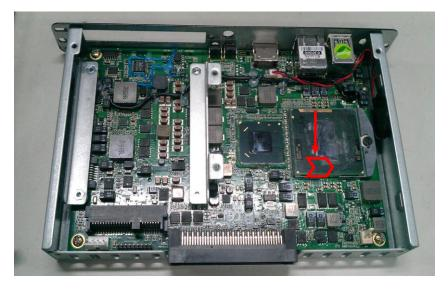
Step 2.2 Insert the CPU in to the slot. Please follow the indication on CPU as mark and slot to ensure the proper insertion of the CPU
