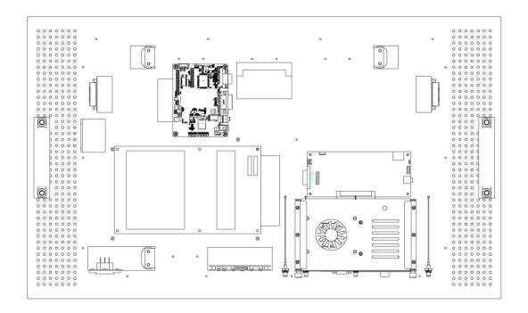
The digital signage OPS870-HM series prototype is based on a 32" display panel with the functional blocks illustrated in Figure 18. It is mainly a 3-board partitioning design consisting of the pluggable module, docking board and the panel control board.
