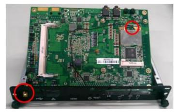
> The wireless Module with two antennas application:
