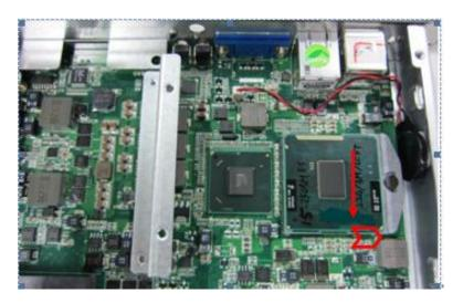
Step 2.3 CPU is inserted into the socket and the latch is closed.
