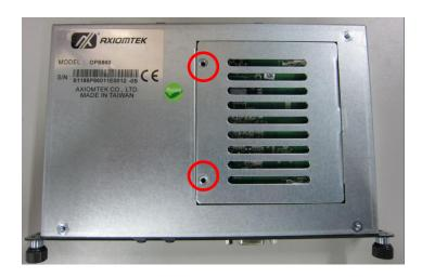
Step 3.2 After losing the screws, extract the real of chassis out of the module.
