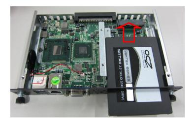
Step 5.4 Pull the HDD Mylar to slot-out the HDD drive
