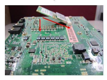
Step 4.3 Find the Antenna cable and connect it wireless LAN card.
