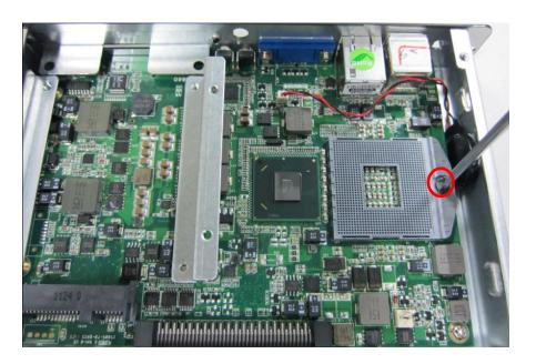
Step 2.2 Insert the CPU in to the slot. Please follow the indication on CPU as mark and slot to ensure the proper insertion of the CPU
