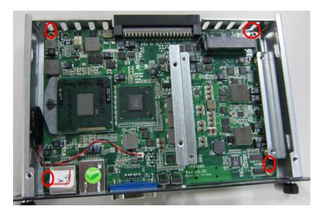
**Step 2 Install CPU**Step 2.1 Loosen the screws of CPU socket
