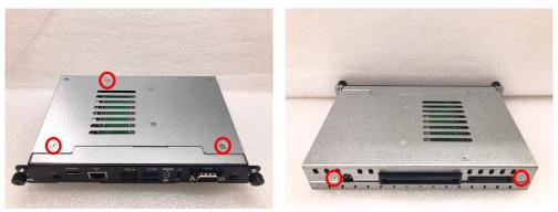
Step 2 Slide the bottom chassis out of the module, and locate the SO-DIMM socket on the board.
