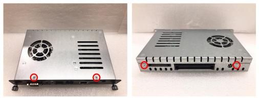
Step 2 To open the upper case, please hold the system with your middle fingers at the Lock Hole, and put your thumbs at the edge of the front panel, then use your thumbs press enough force at the edge of the front panel (① red arrow in the second figure below), meanwhile; lift up the upper case with your middle fingers (② blue arrow in the second figure below).
