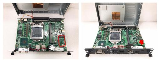
Step 4 Then secure the M.2 2230 Key E Wi-Fi Module to the carrier by tightening up the one M3\*4L pan head screw to the marked position.
