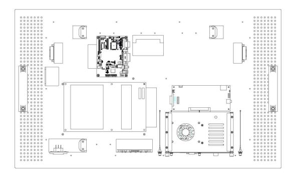
The digital signage OPS700-520 Series prototype is based on a **32**" display panel with the functional blocks illustrated. It is mainly a 3-board partitioning design consisting of the pluggable module, docking board and the panel control board.
