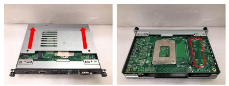
Step 3 Holding the M.2 2280 Key M SSD card at a 30 degree angle up from horizontal, slowly insert the golden fingers into the M.2 2280 Key M slot until it is fully inserted in. And secure the M.2 2280 Key M SSD card to the carrier by tightening up the one M3\*4L pan head screw to the marked position.
