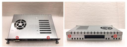
Step 2 To open the upper case, please hold the system with your middle fingers at the Lock Hole, and put your thumbs at the edge of the front panel, then use your thumbs press enough force at the edge of the front panel (①red arrow in the second figure below), meanwhile; lift up the upper case with your middle fingers (②blue arrow in the second figure below).
