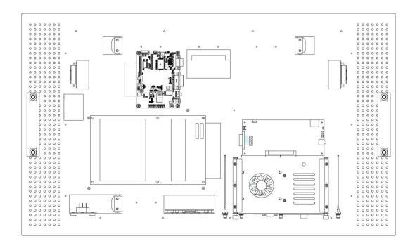
The digital signage OPS500-520-H Series prototype is based on a **32**" display panel with the functional blocks illustrated. It is mainly a 3-board partitioning design consisting of the pluggable module, docking board and the panel control board.
