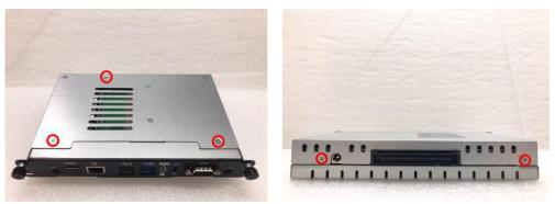
Step 2 Slide the bottom chassis out of the module, and locate the SO-DIMM socket on the board.
