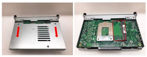
Step 3 Place the memory module into the socket and press it firmly. The socket latches are levered upwards and clipped on to the edges of the SO-DIMM.
