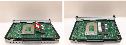
2.1.2 DDR4 SO-DIMM DRAM Installation (SO-DIMM 2)
