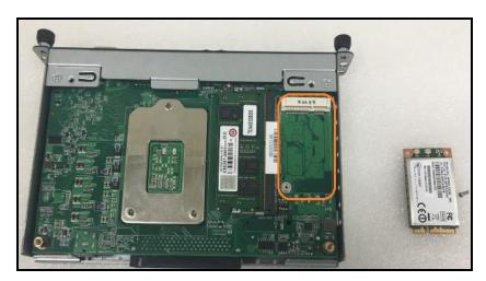
Step 4 Please insert the module then fasten screw carefully.
