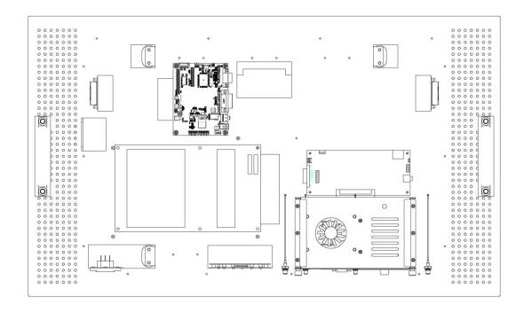
The digital signage OPS500-501-H series prototype is based on a 32" display panel with the functional blocks illustrated. It is mainly a 3-board partitioning design consisting of the pluggable module, docking board and the panel control board.
