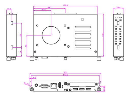
\*While plugging the OPS module, please make sure the heat sink side of OPS module toward the outside. Axiomtek will be out of reasonability if there is any damage occurred due to it.
