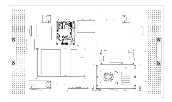
The digital signage OPS500-501 series prototype is based on a 32" display panel with the functional blocks illustrated. It is mainly a 3-board partitioning design consisting of the pluggable module, docking board and the panel control board.
