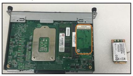
Step 3 Please find the position of Mini PCle slot on the bottom side of OPS.
