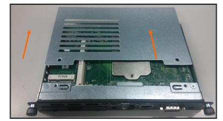
Step 2 After losing the screws, extract the real of chassis out of the module.
