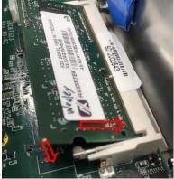
**Step 5** After installing the memory modules, close the cover back onto the system and fasten all screws.
