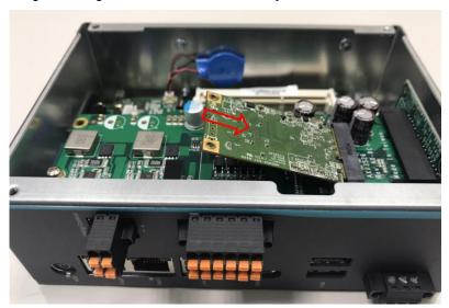
**Step 6** Fix the mSATA storage onto the board with one screw.
