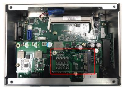
Step 5 Hold the mSATA storage at 30 degrees up from the horizontal direction and inset the golden finger into the slot until it is fully inserted.
