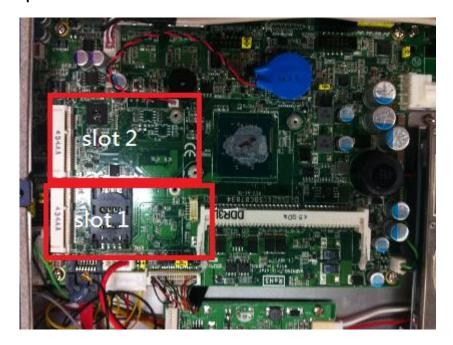
Step 2 Insert the wireless LAN card to the slot. Screw it firmly on the slot.
