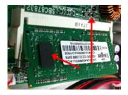
Step 3 Install the memory module into the socket and push it firmly down until it is fully seated. The socket latches are levered upwards and clipped on to the edges of the DIMM.
