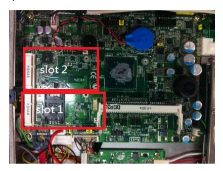
Step 2 Insert the mSATA card to the slot 2. Screw it firmly on the slot.
