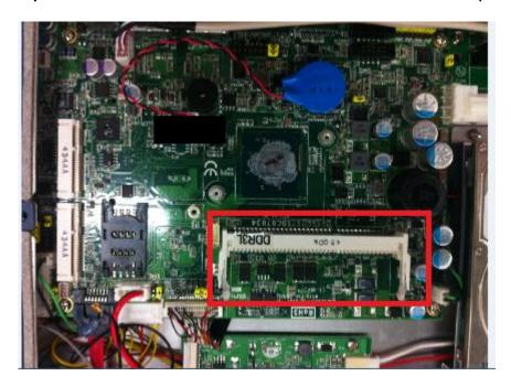
Step 2 Insert the DRAM to the DIMM socket, and then push it down firmly until it is clipped by the socket.
