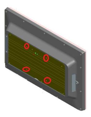
Step 2 Assemble the desktop stand to the chassis, and fix the screws.
