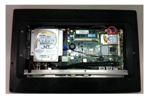
Step 4 There are two connectors on wireless LAN card. One is MAIN, and the other is auxiliary. Connect antenna cable to MAIN connector on wireless LAN card.
