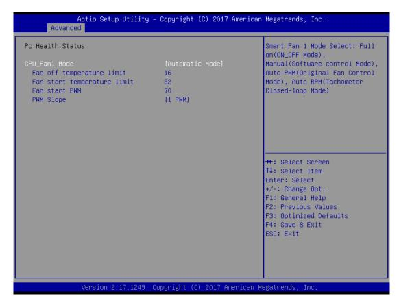
Follow super I/O IT8786 integrated automatic mode as the below to adjust the fan speed.
