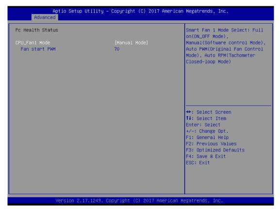
Input the Fan Start PWM to start the fan.
