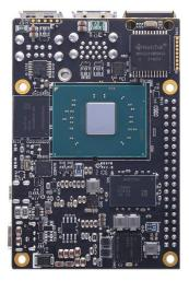
The KIWI310 is a credit card size board with Intel<sup>®</sup> Celeron<sup>®</sup> N3350 processor that deliver outstanding system performance through high-bandwidth interfaces, multiple I/O functions for interactive applications and various embedded computing solutions.
