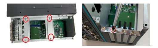
**Step 2** Align the PCI or PCIe card with the slot, press the card into the slot until it is firmly seated and screw it.
