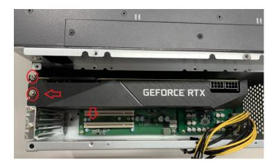
**Step 4** Plug two graphics cables into AX98268 power board and graphics card.
