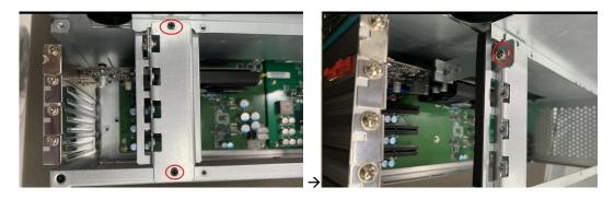
**Step 8** Close the cover back to the chassis and fasten all screws. The installation is complete.
