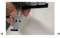
**Step 7** Fasten the first holder bracket in the chassis, adjust the screw position of the extension bracket to fix the add-in card, and then screw it.
