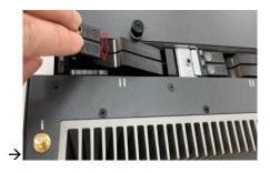
**Step 6** Screw the bracket. The installation is complete.
