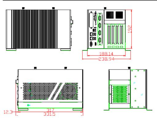
The following diagrams show you the system dimensions with external fan module.
