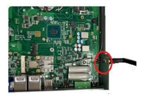
Note:Please use the supplied extended bracket when using a half-size Mini card.
