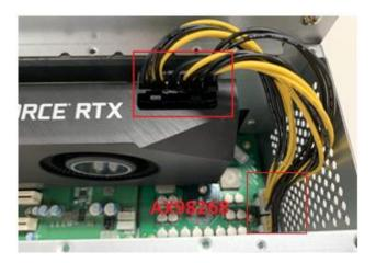
Step 5 Fasten the holder bracket in chassis.
