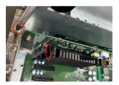
**Step 3** Fasten the below bracket in chassis with standard height (111mm) add-in cards.
