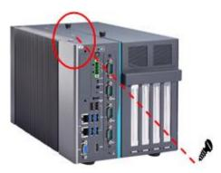
**Step 4** Insert the wireless LAN card into the slot and push it down firmly. Then screw the card tightly to the mainboard.
