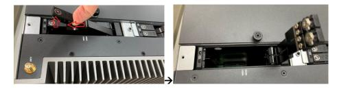
Step 5 Align the connector of the HDD/SSD with the SATA slot of main board. Then, insert the HDD into the HDD tray.
