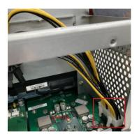
**Step 3** Align gaphics card with the slot, press the card into the slot until it is firmly seated and screw it.
