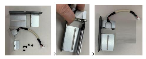
Step 5 Insert the USB stick into the USB dongle kit and screw it.
