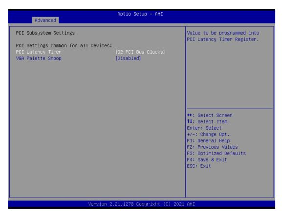
PCI Latency Timer Set the value to be programmed into PCI Latency Timer Register. VGA Palette Snoop Enables or Disables VGA Palette Registers Snooping.
