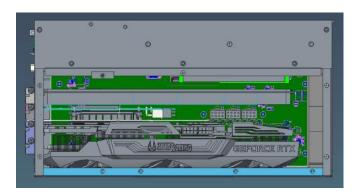
**Step 3** Take the holder bracket and its screws out of the accessory box, then fasten the holder bracket to the chassis to secure the add-on card in place.
