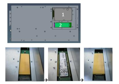
**Step 5** Screw the bracket with 2 screws. Installation is complete.
