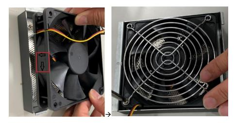
**Step 6** Screw the fan module to the system chassis and plug the fan cable to the fan connector on the riser.
