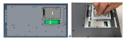
**Step 4** Take the NVMe bracket, thermal pads and its screws from the accessory box and stick a thermal pad on socket, then insert the SSD into the socket (#2) and screw it. Stick another pad on SSD.
