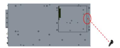
**Step 2** Take the SSD/HDD bracket and its screws from the accessory box, then screw the SSD/DD to the bracket.
