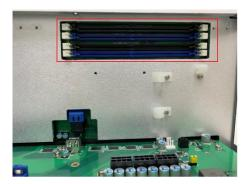
**Step 5** After installing the memory module, close the side cover back to the chassis and fasten all screws. The installation is complete.
