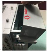
**Step 5** Unscrew the fan bracket, fasten the fan module into expansion box and plug two cables to two connectors.
