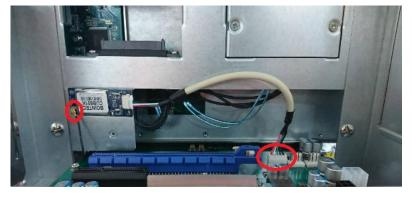
**Step 9** Close the cover back to the chassis and fasten all screws. The installation completed.
