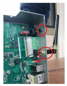
**Step 5** Unscrew the thumbscrew and separating the cover from the expansion box
