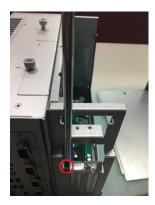
**Step 7** Align the PCI or PCIe card with the slot, press the card into the slot until it is firmly seated and screw it.
