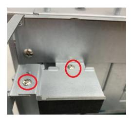
**Step 9** Close the cover back to the chassis and fasten all screws.
