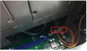
**Step 6** Locate the PCI or PCIe slots and remove the slot bracket which you want to add the card in.
