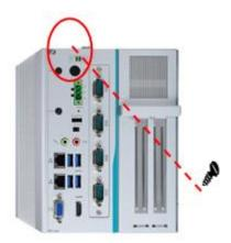
**Step 4** Insert the wireless LAN card to slot. Push it down firmly. Then screw tightly the card to the mainboard
