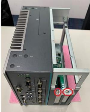
**Step 5** Align the PCI or PCIe card with the slot, press the card into the slot until it is firmly seated and screw it. Then, plug the graphics card power cable.
