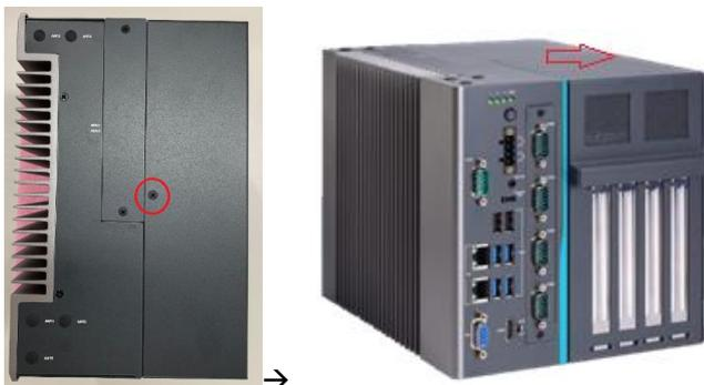
**Step 4** Locate the PCI or PCIe slots and remove the slot bracket from the slot in which you want to add the card.
