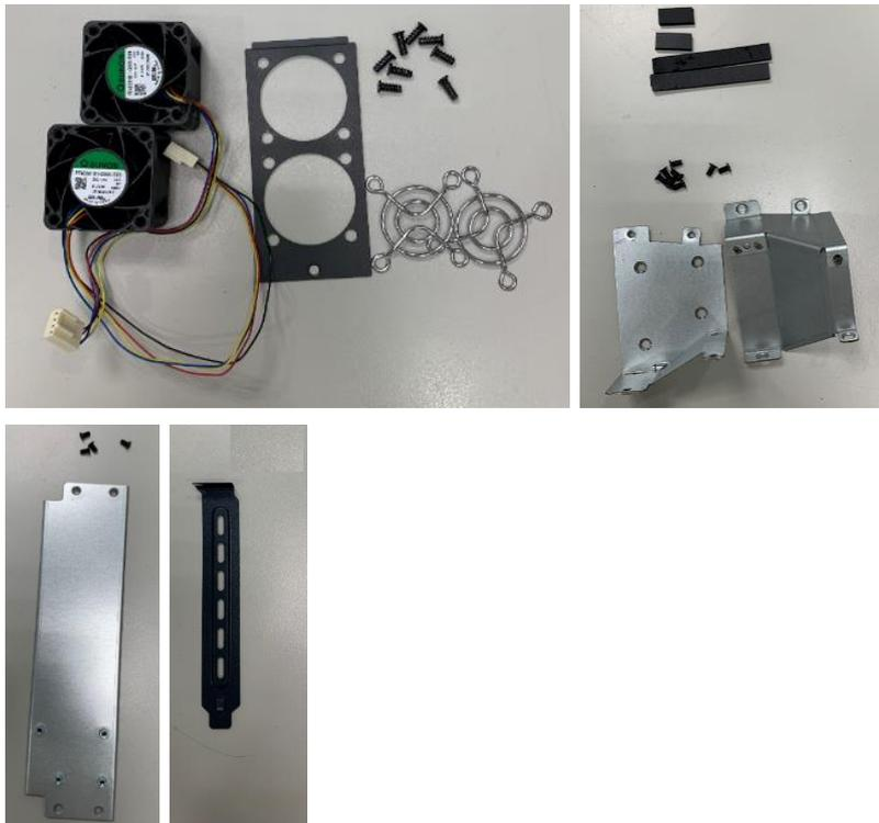
**Step 3** Screw the eight screws into fan and fan bracket.
