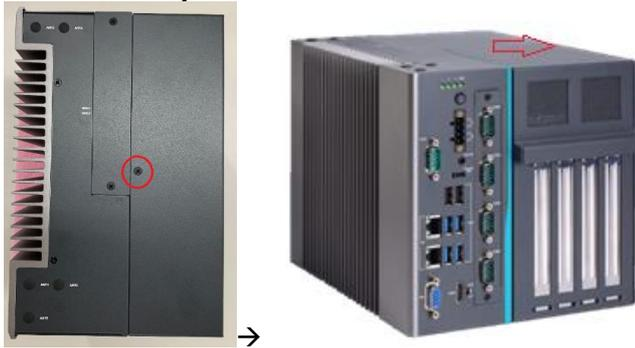
**Step 5** Unscrew the bracket, fasten the fan module into the expansion box and plug cable(s) to connector(s).
