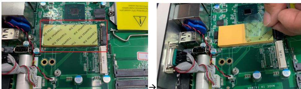
**Step 6** Insert the SSD card to slot and push it down firmly. Then screw the card tightly to the mainboard.
