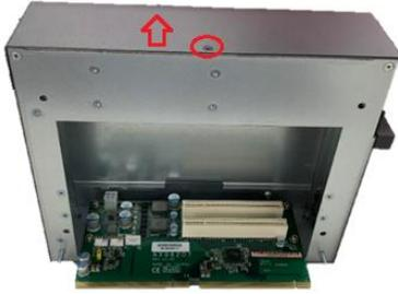
**Step 5** Align the PCI or PCIe card with the slot, and press the card into the slot until it is firmly seated and screw it.
