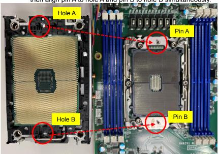
Step 4 Place the CPU cooler module on the CPU socket on the motherboard, and then align pin A to hole A and pin B to hole B simultaneously.
