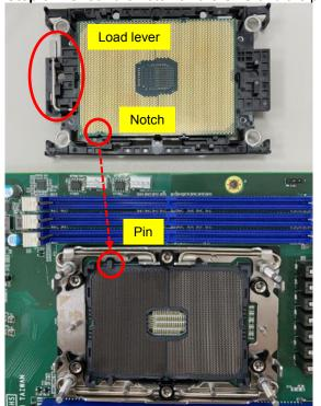
**Step 3** Check the notch on the CPU and the pin on the CPU socket of IMB700.
