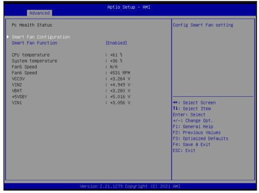
This screen displays the temperature of system and CPU, cooling fans speed in RPM and system voltages (VCC3V, VIN2, VBAT, +5VSBY and VIN1).
