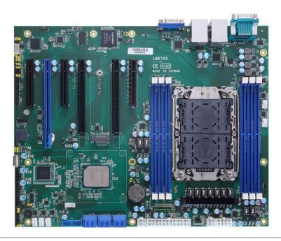
The IMB700 is an advanced ATX industrial severboard based on the Intel® Xeno® Scalable Ice Lake-SP processors in an LGA4189 socket, and comes with an Intel® C621A chipset. Featuring enhanced computing power to deliver optimal computing and visual performance, the IMB700 motherboard is an ideal solution for developing major industry applications ranging from financial modeling to deep learning AI and video surveillance.
