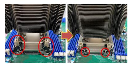
**Step5** Put the fan module on the CPU cooler and tighten two screws (8in-LBF).
