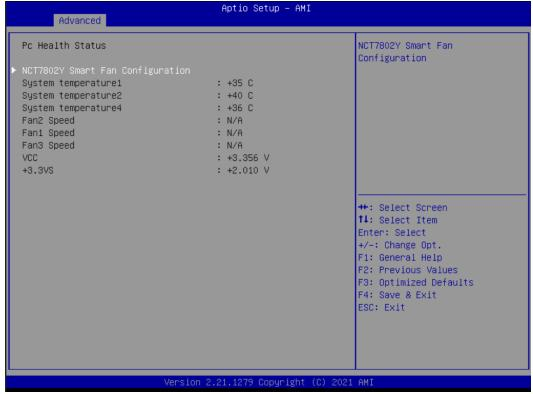
This screen displays the temperature of system, cooling fans speed in RPM and system voltages.
