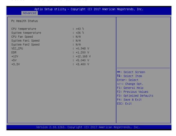
This screen displays the temperature of system and CPU, cooling fans speed in RPM and system voltages (VCC\_CPU, DDR, +12V, +5V and +3.3V).
