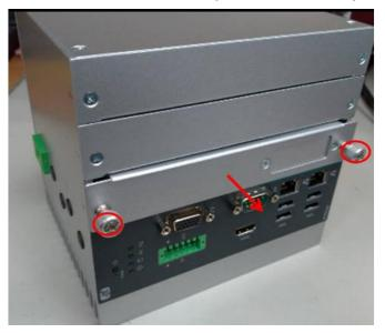
Step 3 Fasten the SSD screws (marked by the red arrows below) to fix the SSD. Then screw the SSD firmly to the tray (marked by the yellow circles) and install the tray back to the system.
