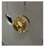
Step 4 Hold the other side and screw the antenna.
