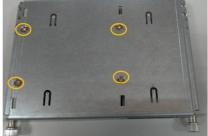
Step 4 Loosen the screws to open the CFast door and install the SIM and CFast card, as illustrated below. Then lock the CFast door back to the system.
