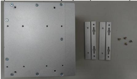
Step 2 Assemble the bracket to the system and fasten screws tight.
