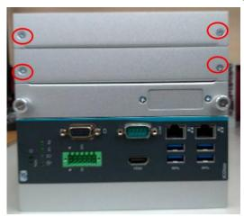
Step 3 Install the module card as shown below, and fasten the screws firmly to finish the installation.
