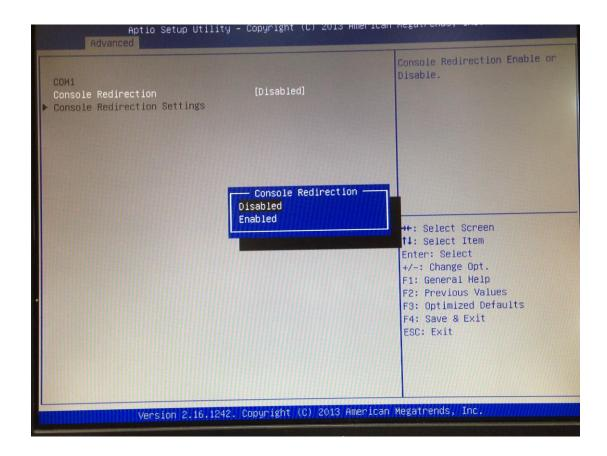
If the setting for the console redirection function is changed for [Enabled], the settings specify how the host computer and the remote computer (which the user is using) will exchange data. Both computers should have the same or compatible settings.
