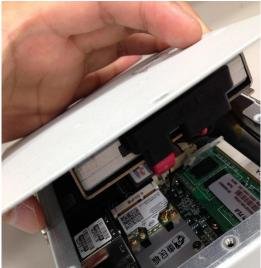
Step 6 Put the cover back to the system, and fasten screws tight close the chassis.
