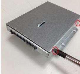
Step 4 Put the HDD bracket on the cover and use 4pcs screws to fix tightly. Takes the HDD SATA+Power HDD cable and Cable Tie out from the accessory bag and connect SATA+Power HDD cable to HDD then use Cable Tie to fix it on the HDD bracket, cut off the lengthy Cable Tie.
