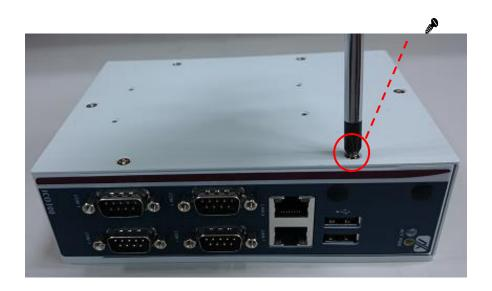
Step 3 Loosen 4pcs screws of the cover, and put the HDD into the HDD bracket and fix the HDD by 4pcs of screws in the accessory bag.
