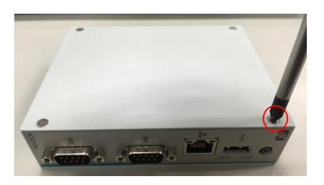
Step 3 Following(Figure 3-1) push the SIM slot back to unlock SIM slot, inserting the SIM card and put it back(Figure 3-2), and lock the SIM slot(Figure 3-3).
