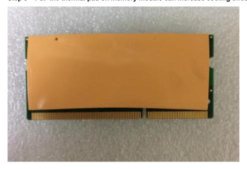
Step 4 Use two fingers to hold the memory module, and insert the gold figure into the slot and push the module down.
