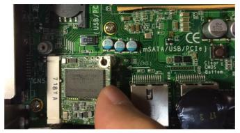
Step 4 Fasten the screw tightly.
