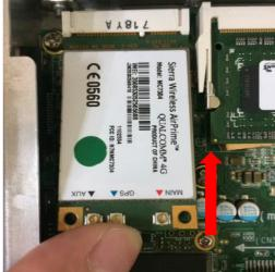
Step 5 Insert the 3G module and screws it tight.
