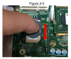
Step4. Insert the wireless module into the slot which marking with "USB/PCIe".
