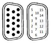
Note: Speaker-out and line-out are shared on the same connector but it's either one functionality, line-out is the highest priority, if pin#7 is connected and detected the signal of line-out, signal is switching to line-out.
