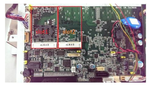
Step 2 Insert the wireless LAN card to the slot. Screw it firmly on the slot.
