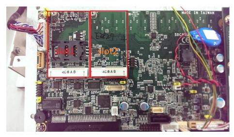
Step 1 Open the back cover and find out the mini-card slot on main board.
