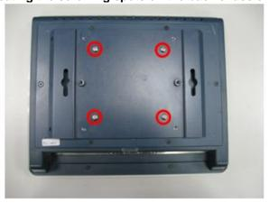
Assemble the VESA-ARM to the back chassis, and fix them to the Step 2 GOT5152T-845 with screws (see Figure 2-18).
