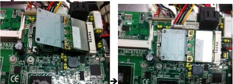
Step 3 Locate the built-in antenna cable and connect it to the wireless LAN card. There are two connectors on the wireless LAN card. One is the main connector whereas the other is the secondary connector. The main connector on the wireless LAN card is the one to be connected to the antenna cable (see Figure 2-11).
