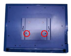
Step 2 Assemble the desktop stand to the back chassis, and fix them to the GOT5152T-8485 with screws (see Figure 2-16).
