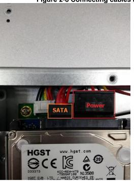
Figure 2-8 Connecting cables to connectors
