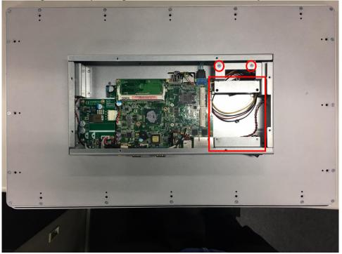
Figure 2-5 Separating the bracket from the HDD tray
