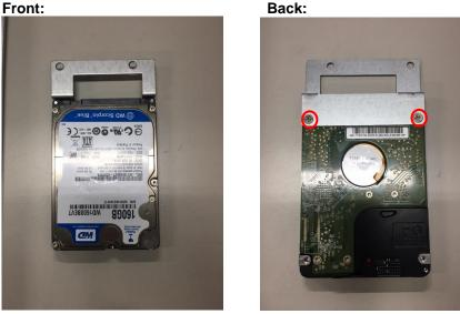
Figure 2-6 Fastening a HDD to the bracket
