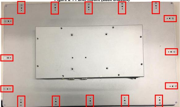
Figure 2-1 Panel mount (back chassis)
