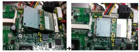
Step 3 Locate the antenna cable and connect it to the wireless LAN card (see Figure 2-13).
