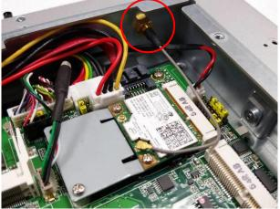
Figure 2-15 Antenna outlet (external view)
