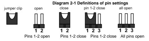
Before applying power to GOT3217WL-845-PCT, please make sure all of the jumpers and connectors are in default position as listed in Table 2-1.
