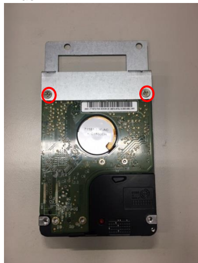
Figure 2-6 Fastening a HDD to the bracket
