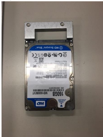
Figure 2-6 Fastening a HDD to the bracket
