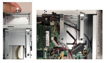
©Copyright 2020 Axiomtek Co., Ltd. Version A1 Sep 2020 Printed in Taiwan Step 5Take 2.5" HDD on the bracket and fasten the four screws in<br/>the other side. And plug the "SATA + Power" connector to<br/>complete the installation. Completing installation by
