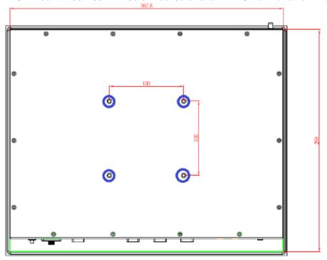
**Wall mount:** This is an optional wall kit. Screw it on the rear of chassis to support wall mount.
