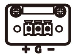
NOTE: The safety ground must be connected to ensure the unit working appropriately.
