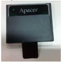
Step 3 Insert the card into the socket.
