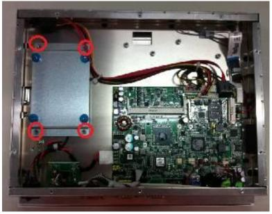
Step 3 Fix the HDD on bracket by 4 screws.
