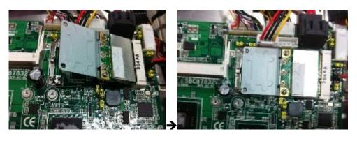
Step 3 Find the Antenna cable and connect it on wireless LAN card.
