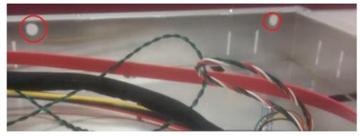
Step 4 Remove the antenna plug from the top of back cover, then Install the antenna on the antenna connector.
