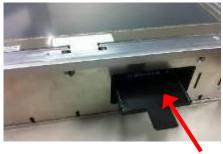
Step 4 Close the cover of CFast<sup>™</sup> card slot and fix it. Installation completes.
