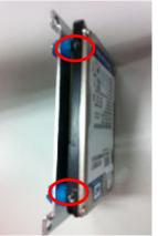
Step 4 Fix the HDD bracket into the system, and plug the data and power cable to HDD & SBC87834 mother board. Installation completed.
