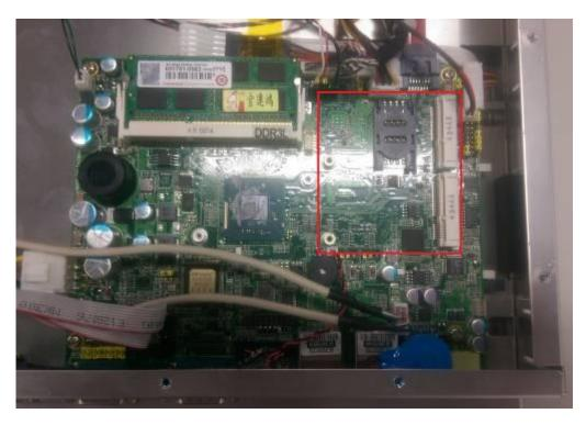
Step 2 Insert the wireless LAN card to the slot. Push it down firmly until it is clipped by the slot.
