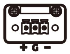
NOTE: The safety ground must be connected to ensure the unit working appropriately.
