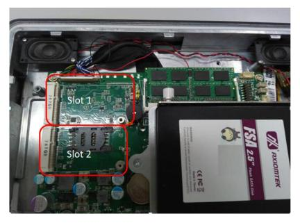
Insert the mSATA card into the slot 1. Screw it firmly on the slot. Step 2
