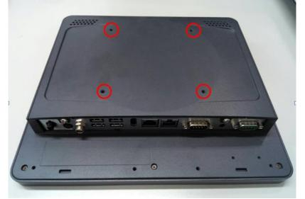
Step 1 Find out the holes as marked on the back side of chassis.
