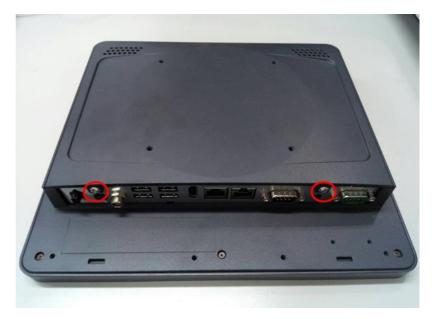
Step 3 Install the 2.5" SSD storage into the red marked bracket.
