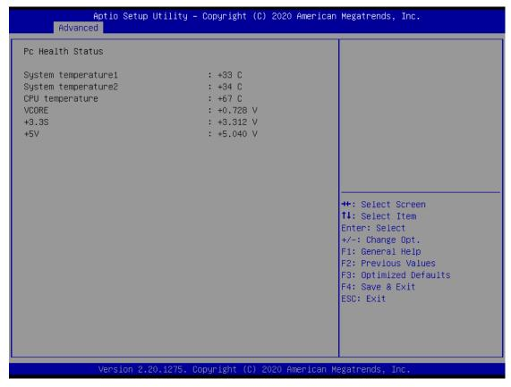
This screen displays the temperature of the system and CPU as well as system voltages (VCORE, +3.3V, +12V and +5V).
