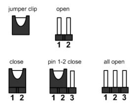
Properly configure jumper settings on the CAPA500 to meet your application purpose. Below you can find a summary table of all jumpers and onboard default settings.
