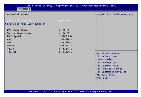
This screen displays the temperature of CPU and system, cooling fan speed in RPM, standby and system voltages (+3.3VSB/+5VSB and +3.3V/+5V).
