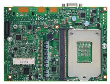
The CAPA500, a high performance 3.5" board, supports LGA1151 socket for  $6^{th}/7^{th}$  Generation Intel® CoreTM i7/ i5/ i3 processors with H110 (Q170 optional) chipsets. The board delivers outstanding system performance through high-bandwidth interfaces, multiple I/O functions for interactive applications and various embedded computing solutions.
