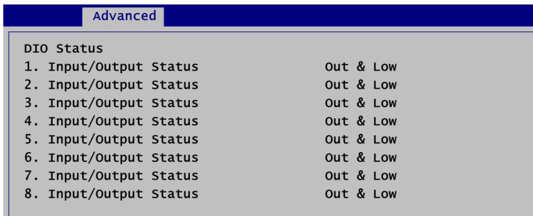
Once it is enabled, you can load manufacture default and access to the DIO status sub screen to set output or input, see image below.
