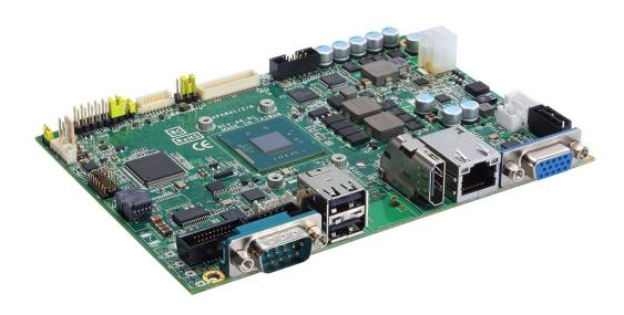
The CAPA848, a 3.5" board, supports Intel<sup>®</sup> Celeron<sup>®</sup> N2807 processor. It delivers outstanding system performance through high-bandwidth interfaces, multiple I/O functions for interactive applications and various embedded computing solutions.
